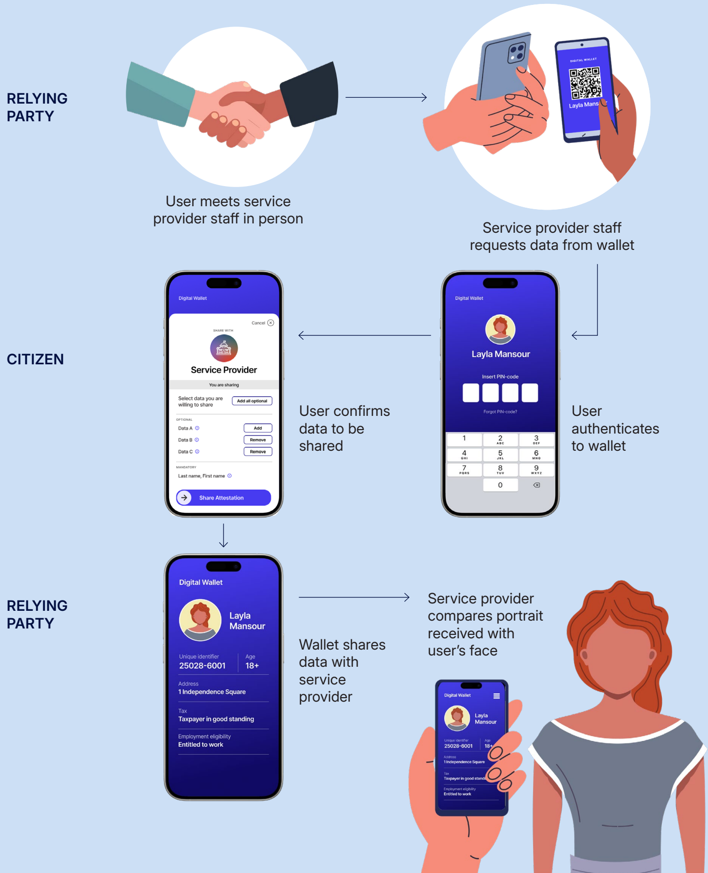
FIGURE 5. Using a digital wallet to access services in person (indicative transaction flow)
